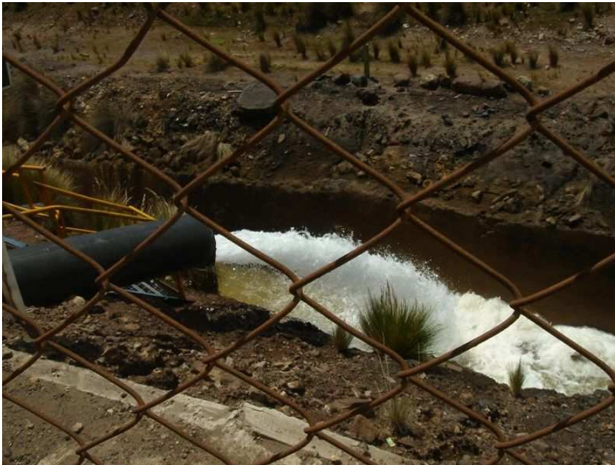
Mine wastewater effluent with neutralized pH from tailing runoff, Peru
