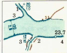
495. Shore with built-up but not reinforced slope \_\_\_\_\_
