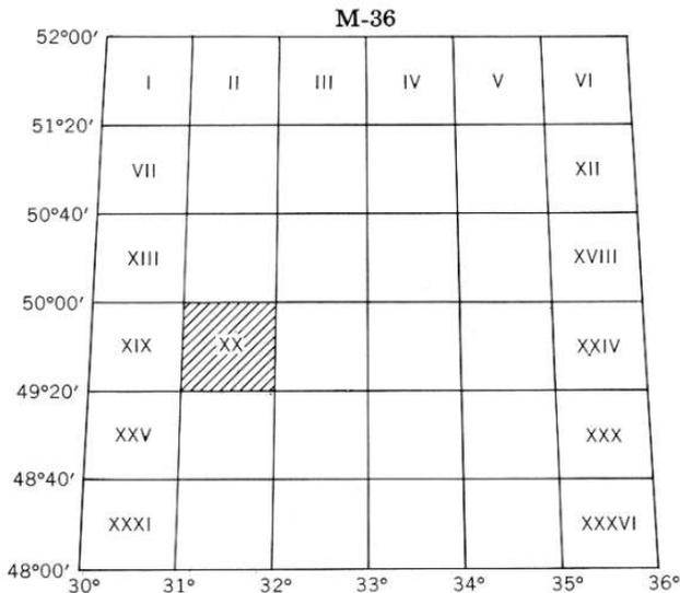
FIGURE 3. Method 1, 1:200,000 scale division of 1:1,000,000 Sheet M-36.
