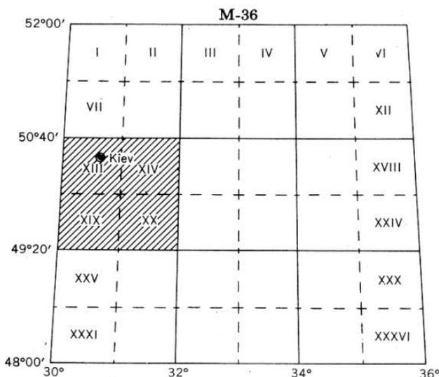
FIGURE 5. Method 3, 1:200,000 Scale division of 1:1,000,000 Sheet M-36.
