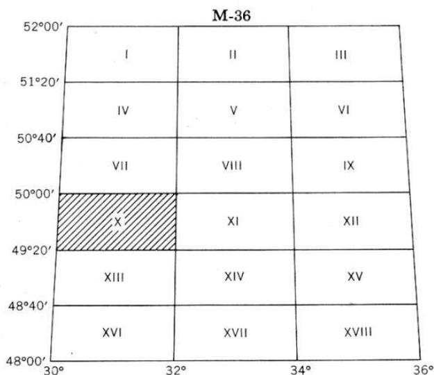
**FIGURE 4. Method 2, 1:200,000 scale division of 1:1,000,000 Sheet M-36.**
